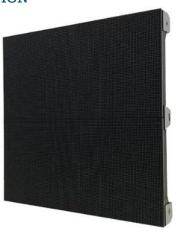
The LIB-LIS Series is the indoor fixed products. Four corners of the box are integrally diecast with the precision capable of meeting the splicing flatness requirements; the profile process is used in the frame, allowing for free change of sizes, meeting different dimension demands of the project. It supports the front and rear installation and maintenance.
